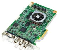
**STORM 3G** is an internal board equipped with 3G-SDI I/O, HDMI monitor out, RS-422 for VTR control and REF In. The incoming baseband signal can be captured in either 10-bit or 8-bit video. Choice of codecs includes uncompressed, Grass Valley HQX (10-bit) / HQ (8-bit), AVC-Intra, and XDCAM compatible MPEG-2. Audio is embedded in both SDI and HDMI, providing high-quality audio I/O. A timecode option is also available enabling linear timecode input as well as two reference outputs.
