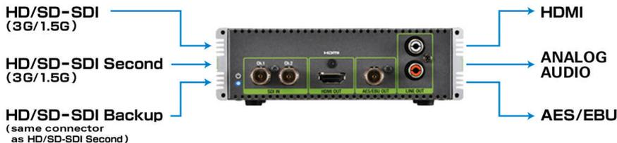
The analog audio and AES/EBU outputs, used for audio de-embedding, are a welcome feature in monitoring situations, for both 2D and 3D content.
