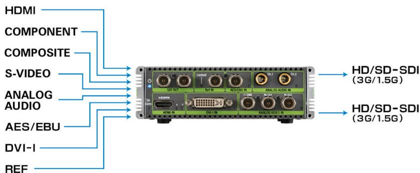
The ADVC G1 will convert and/or upconvert, at the user's choice, sources from HDMI, DVI, component, composite, S-Video, AES/EBU, and analog audio to HD/SD-SDI (3G/1.5G support). With its audio inputs, the ADVC G1 can also be used as an audio embedder. It also features a reference in port which can serve as a frame synchronizer for the analog inputs, eliminating the need to purchase separate expensive equipment.
