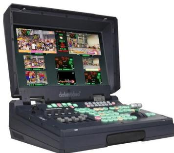
The HS-2000L is a five channel 10-bit HD-SDI full AV switcher. Its DVI-D connection makes it ideal for use with presentation software while the integrated audio mixer with balanced XLR connectors provide four channels of microphone or line audio inputs.
