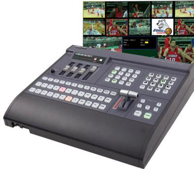
Datavideo SE-600 is an eight input Standard Definition video switcher, with built in dual channel audio mixer. Multi-View output display each input. Other features include audio peak-meter, clock and dual logo store.
